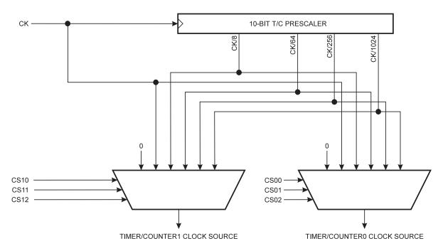
For Timer/Counters 0 and 1, the five different prescaled selections are: CK, CK/8, CK/64, CK/256 and CK/1024, where CK is the oscillator clock. In addition, the Timer/Counters can be stopped.
