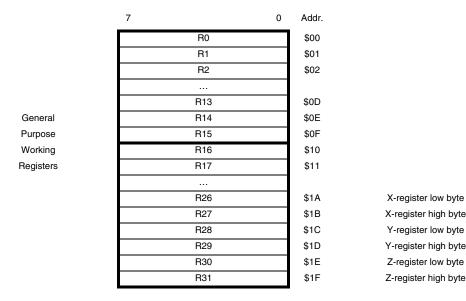
Figure 6. AVR CPU General-purpose Working Registers
