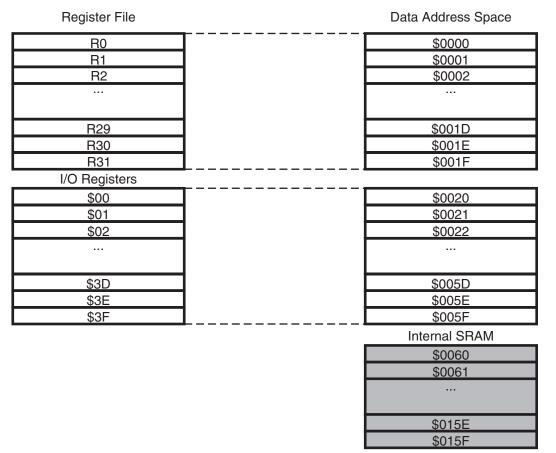
The lower 352 data memory locations address the register file, the I/O memory and the internal data SRAM. The first 96 locations address the register file + I/O memory, and the next 256 locations address the internal data SRAM.
