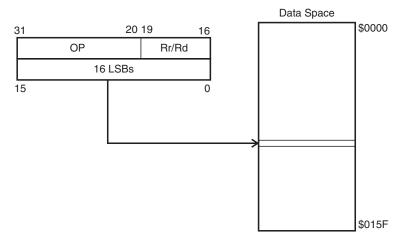
A 16-bit data address is contained in the 16 LSBs of a 2-word instruction. Rd/Rr specify the destination or source register.
