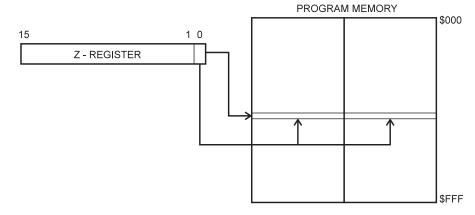
Constant byte address is specified by the Z-register contents. The 15 MSBs select word address (0 - 4K), the LSB selects low byte if cleared (LSB = 0) or high byte if set (LSB = 1).
