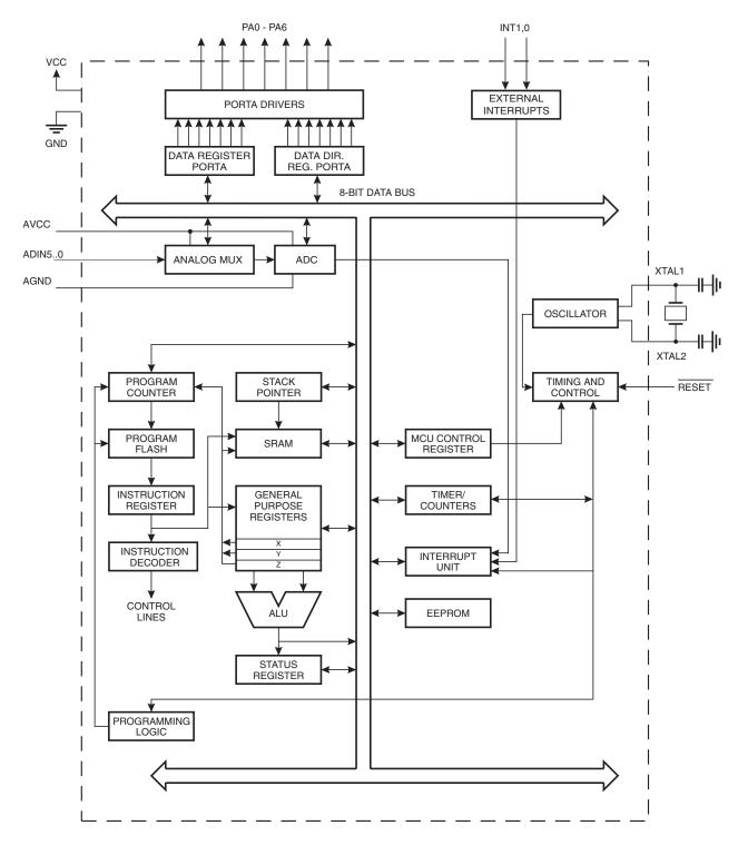
The AVR core combines a rich instruction set with 32 general-purpose working registers. All the 32 registers are directly connected to the Arithmetic Logic Unit (ALU), allowing two independent registers to be accessed in one single instruction executed in one clock cycle. The resulting architecture is more code efficient while achieving throughputs up to ten times faster than conventional CISC microcontrollers.
