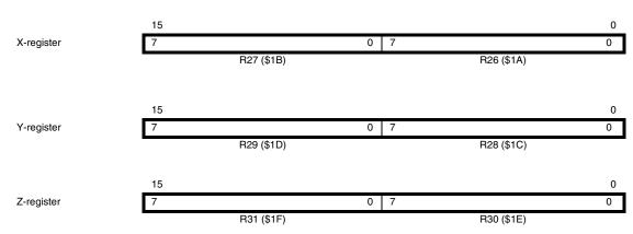
Figure 7. X-, Y- and Z-registers
