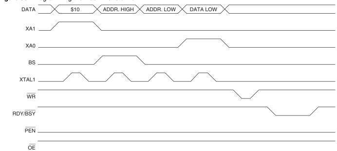
Figure 36. Programming the Flash Waveforms
